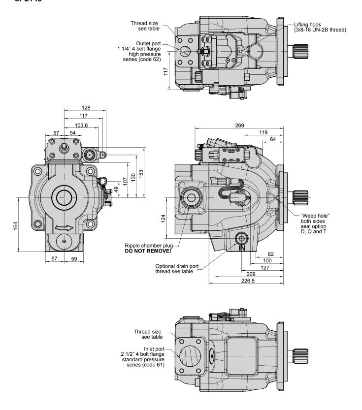
For thru drive dimensions and shaft information please check catalogue MSG30-2800/UK (Axial Piston Pumps - Series P2 / P3.
