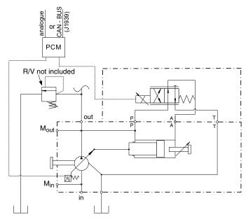
Displacement control with optional pressure limitation (main: D / DP) w/ Parker supplied PCM w/ Pressure Sensor
