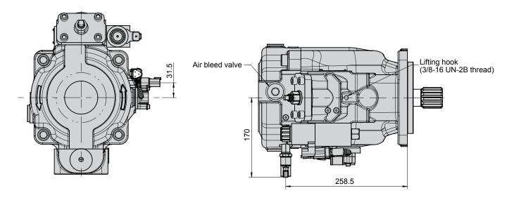
Port option D (pump with metric threads)
