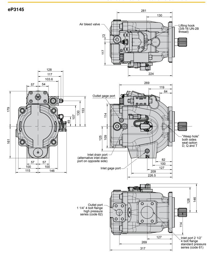
**For thru drive dimensions and shaft information** please check catalogue **MSG30-2800/UK** (Axial Piston Pumps - Series P2 / P3.
